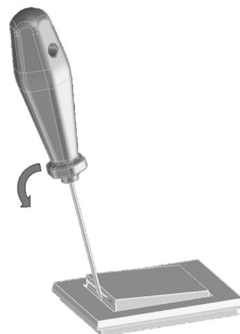
Place a screwdriver in the middle of the open side, between the frame and the room card slot. Release the locking hooks on the cover with a careful lever movement. This can lead to a slight deformation that does not result in damage.
