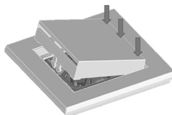
Hold the cover frame in the desired position on the switch and press the locking hooks on the closed side of the cover into the recess provided. By pressing vertically on the cover, it locks into place.
