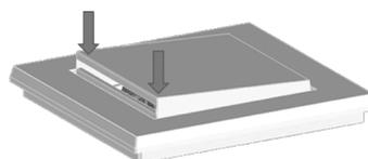
If the closed side is locked, repeat the process with the open side. Use the outer parts of the cover as a pressure point so as not to damage it. This side also clicks into place when you press it vertically.
