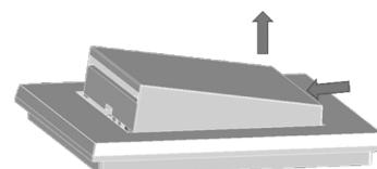
Now press the closed side inwards and pull the cover out of the catch. Also hold the cover frame, as it is no longer fixed after the cover has been removed.
